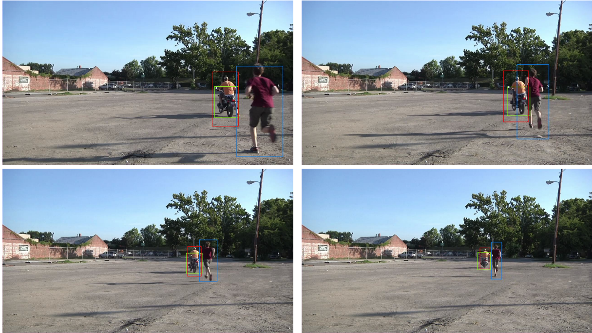
Figure 4: Four frames tracking two people and one motorcycle. Two separate person tracks in red and blue, and the motorcycle track in green. The tracker is robust despite the fact that one person occludes most of the motorcycle, the tracks of the two people overlap, and all three objects become very small as they recede from the camera.
